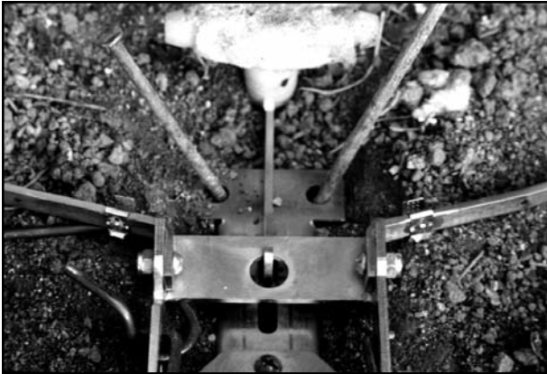
7. Using gutter spikes, firmly anchor the throw mechanism to the ground
